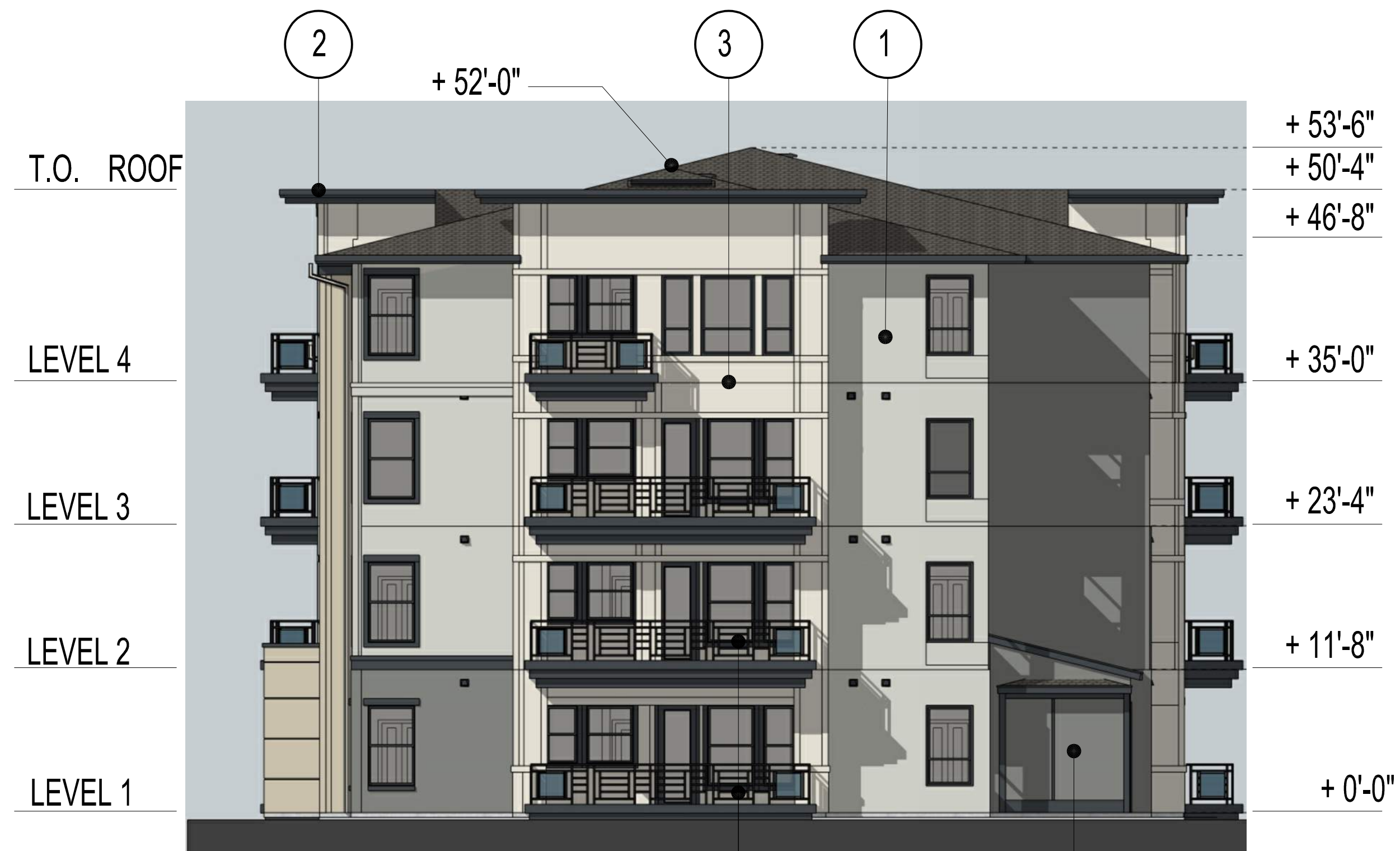
4 BUILDING TYPE 3 - LEFT ELEVATION 1/8" = 1'-0"
