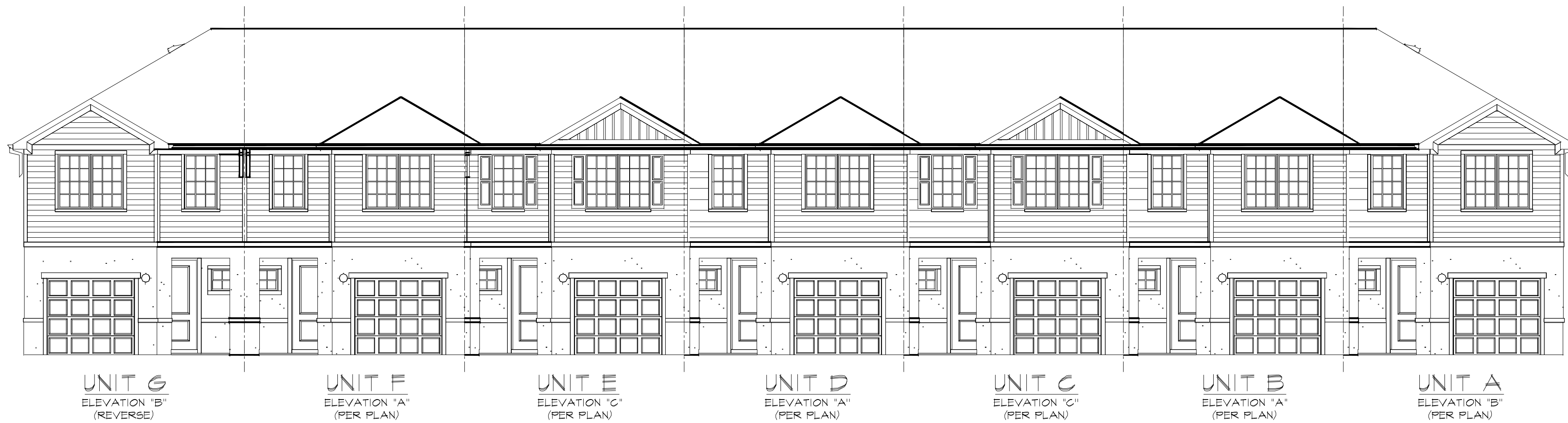
2 B-3 7 - UNIT BUILDING SCALE: 1/8" = 1'-0" MPT07
