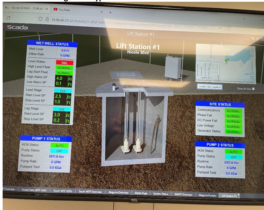
Figure 3: Typical HMI Screen for Lift Station
